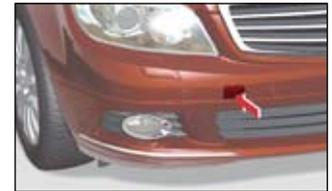
Attachment points for a tow bar/rope, using the C-Class as an example (towing lugs are included in the vehicle tool kit). The specific attachment points for the relevant model are shown in the owner's manual.
