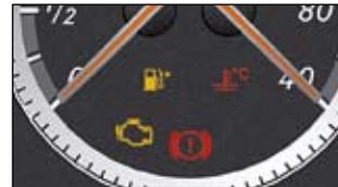
The engine oil and coolant levels are displayed in the instrument cluster. (The owner's manual tells you how to check these)
