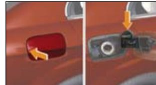
Tyre pressures, incl. spare wheel (the tyre pressure chart is inside the fuel filler flap)
